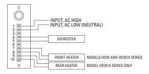
Figure 2. Wiring Diagram for 24/120/230 VAC Models
